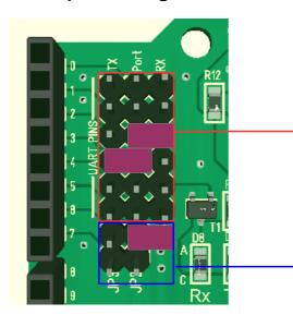
Set the jumpers for the communication ports in the upper left corner as in the picture left. The internal UART on **port**2 and 3 will be connected in this case to the RS485 interface of the shield of the second BUS.
