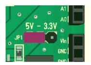
The Arduino UNO works with 5V internally. You have to set this Jumper to the 5V position (for 3.3V boards for example Arduino 101 to the 3.3V position).
