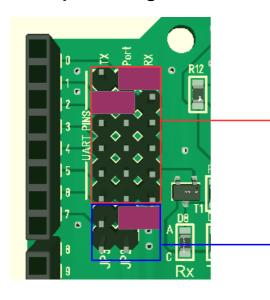
Set the jumpers for the communication ports in the upper left corner as in the picture left. The internal UART on **port 0 and 1 will be connected** in this case to the RS485 interface of the shield of the **first BUS**.
