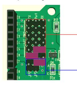
Set the jumpers for the communication ports in the upper left corner as in the picture left. The internal UART on **port**4 and 5 will be connected in this case to the RS485 interface of the shield of the third BUS.
